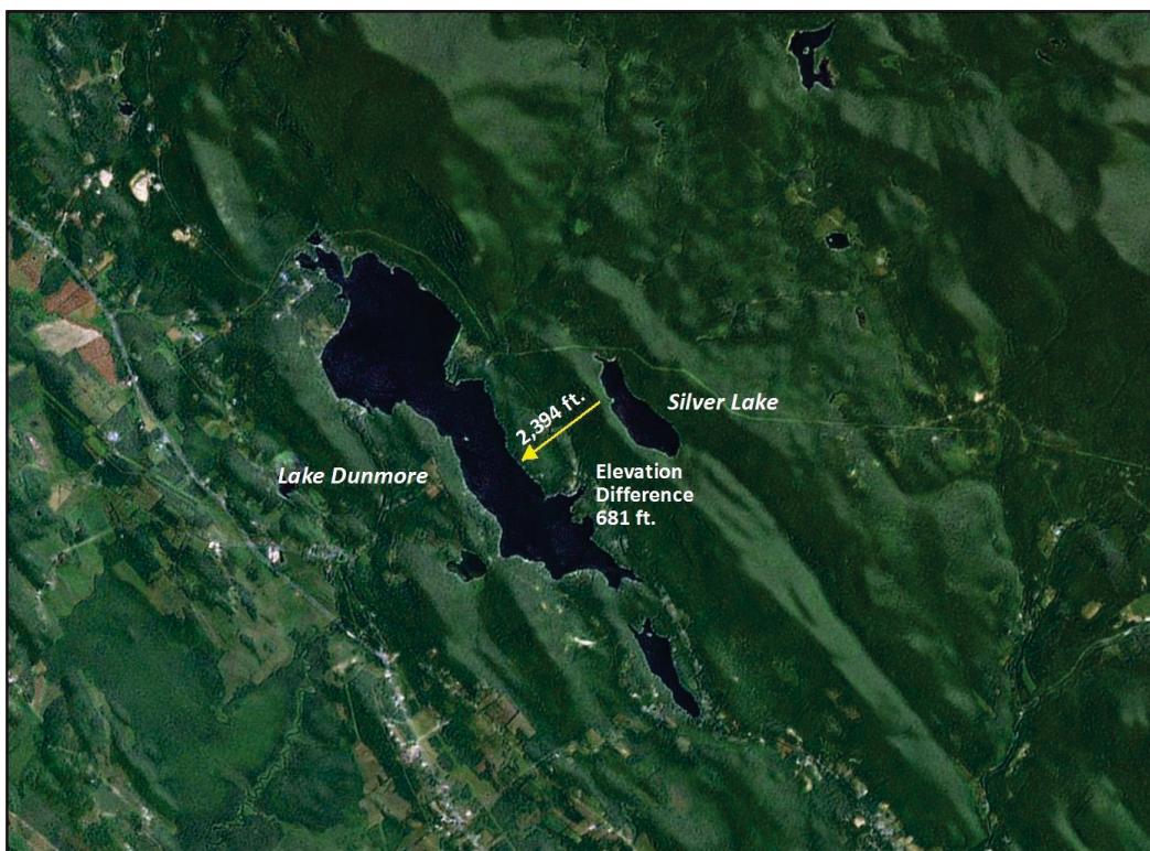
Figure 28. Potential pumped storage configuration between Silver and Dunmore Lakes in Vermont.
