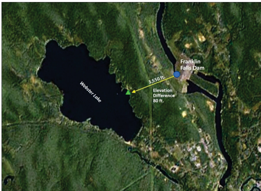
Figure 16. Potential pumped storage configuration at Franklin Falls Dam in New Hampshire.
