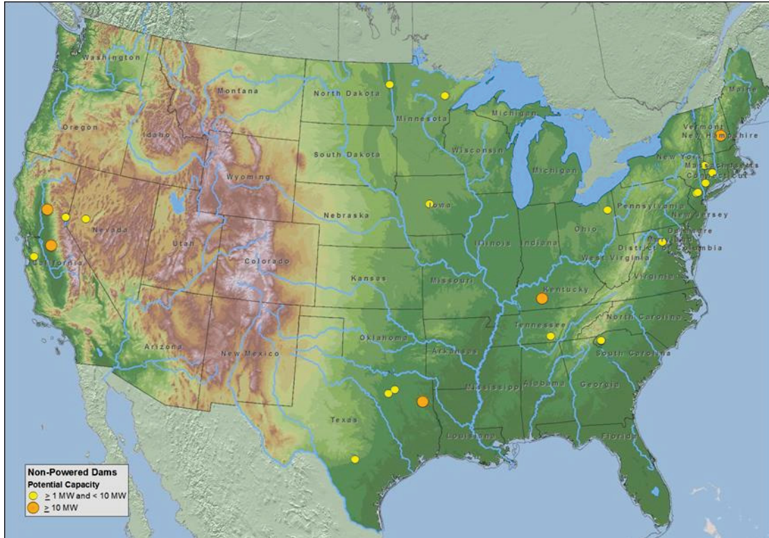
Figure 18. Potential new pumped storage plant sites at existing non-powered dams.
