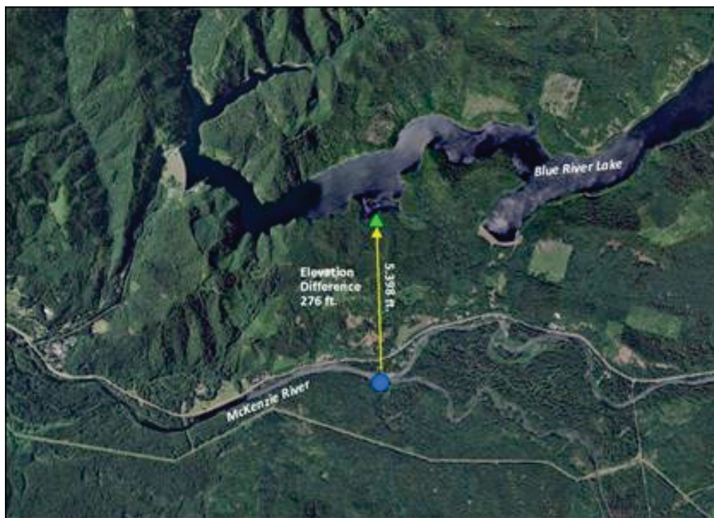
Figure 23. Potential pumped storage configuration on the McKenzie River in Oregon.
