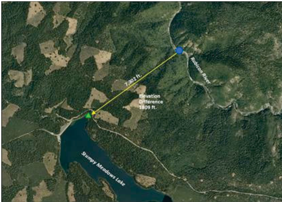
Figure 24. Potential pumped storage configuration on the Rubicon River in California.
