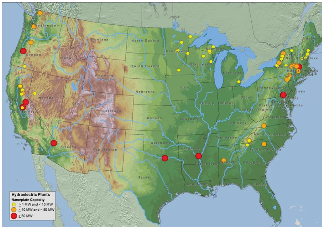
Figure 11. Potential new pumped storage plant sites using existing hydroelectric plants.
